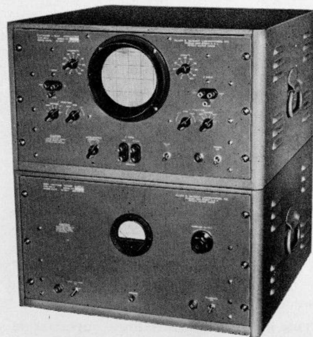
Figure 3. The Type 281-A Cathode-ray Indicator and the Type 286-A High-voltage Power supply, fastened together in their cabinets
