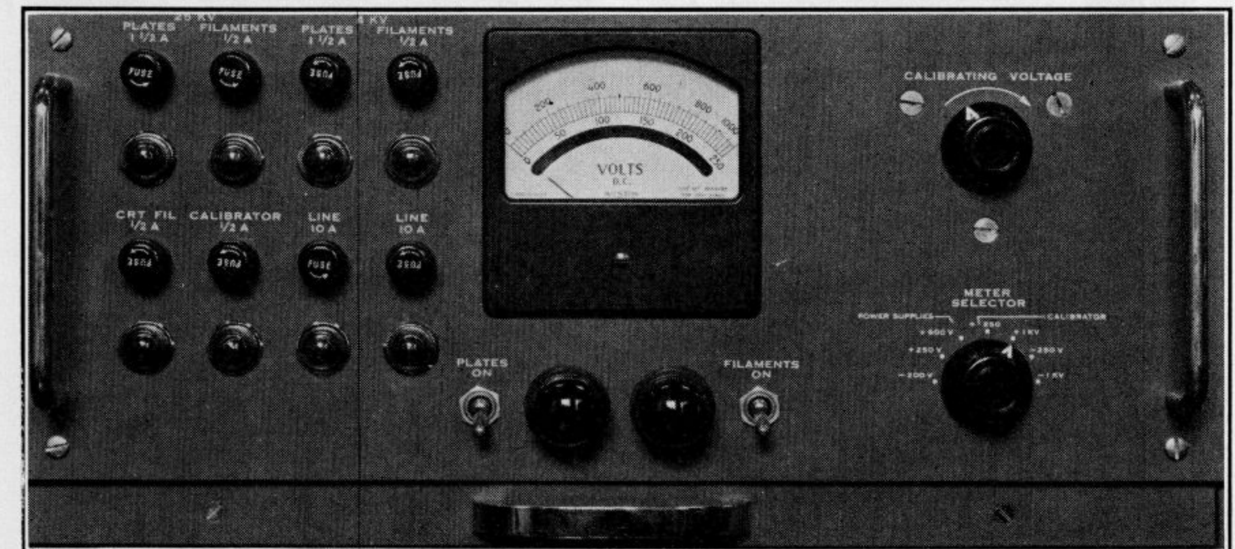
Figure 3. A portion of the control panel of the Type 293 showing the voltage-calibrator controls and meter
