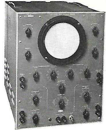
The new Du Mont Type 303-AH is a wide-band, high-gain, quantitative cathode-ray oscillograph that is particularly well suited to the measurement of random, rapid, single transients with low repetition rates. The Type 303-AH features a choice of three accelerating potentials: 3000, 7000 and 10,000 volts.
