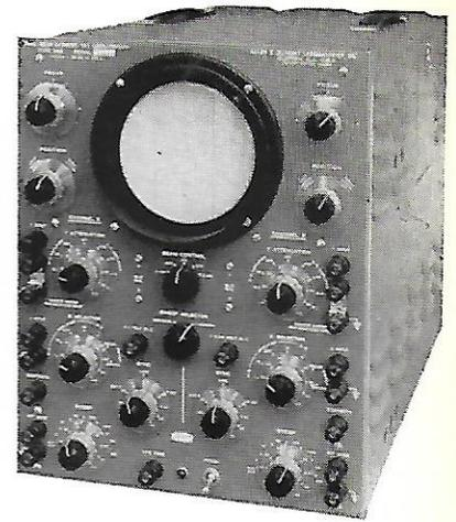
with transparent, skirted knobs afford centralized, finger-tip control. Controls of similar function are mounted on the same axis to give the operator even greater facility in the use of the Type 322. Extra stability is assured by such refinements as the regulated filament supply on Y-input stages. Separate power supplies are employed for each channel.
