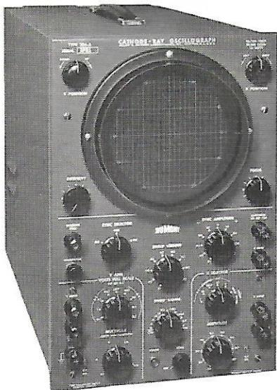
The new Du Mont Type 304-A Cathode-ray Oscillograph, successor to the world-famous Type 304-H, is a true electronic voltmeter, enabling rapid, accurate amplitude measurements of any portion of a 0 to 1000 volt signal within the frequency range of the instrument. The Type 304-A features a sensitivity of 100 millivolts d-c full scale, equivalent to a deflection factor of 25 peak-to-peak millivolts per inch (10 peak-to-peak millivolts/cm), and high gain a-c or d-c amplification.
