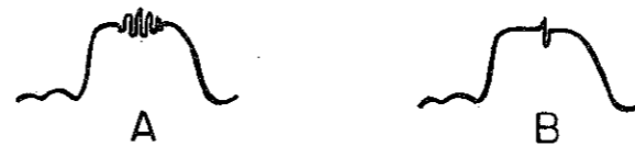
FIG. 44. A video i-f response curve showing excessive marker width at A, and normal marker width at B.
