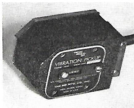
Figure 2. With many transducers, such as this one, it is important that the amplitude range not be exceeded
