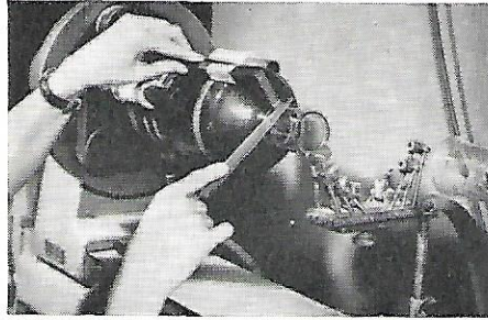
Figure 1. The bulb of the tube to be sealed is mounted in a glass lathe. Here the operator is marking the bulb for cutting of the waste neck.
