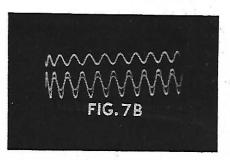
Figs. 7 A & B demonstrate the ability of the switch to handle a square wave as well as to generate one. The setup consists of two electronic switches, the output of one being coupled to one of the inputs of the other. This subtracts one channel and we have left the facilities for three patterns. For easy
