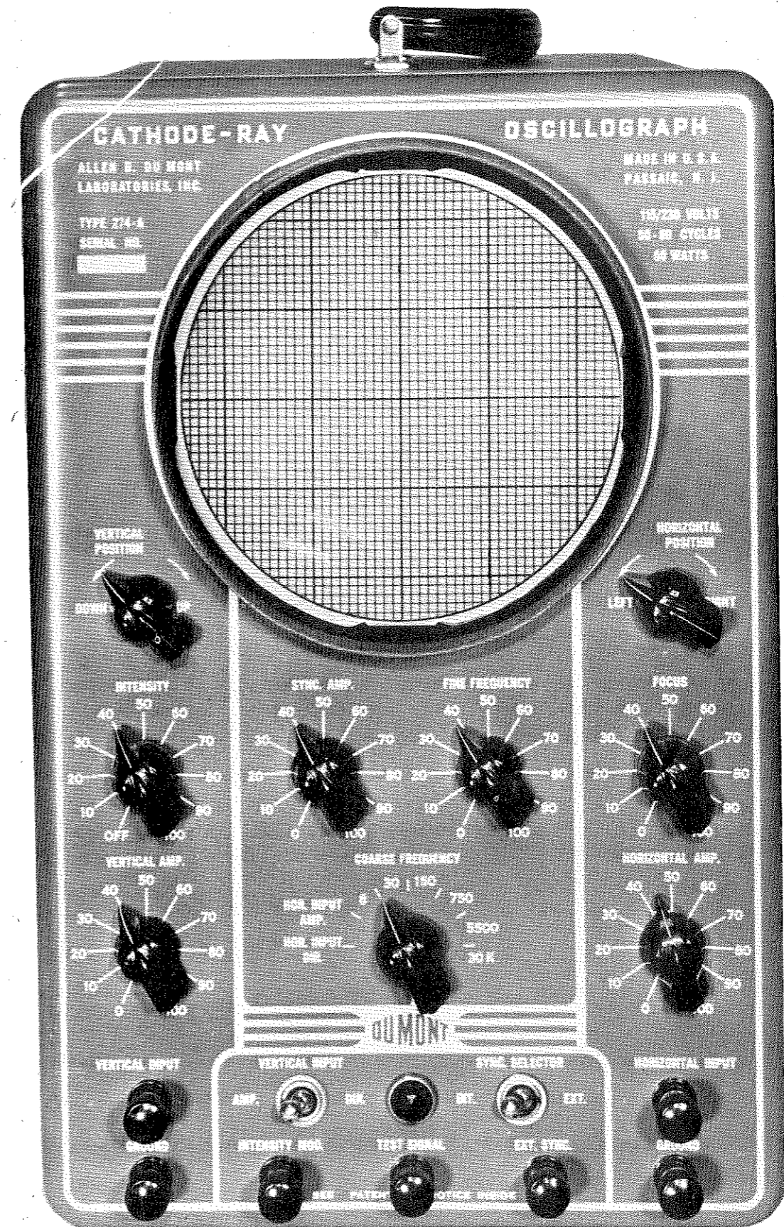
FIGURE 3-3 FRONT PANEL VIEW OF TYPE 274-A CATHODE-RAY OSCILLOGRAPH
