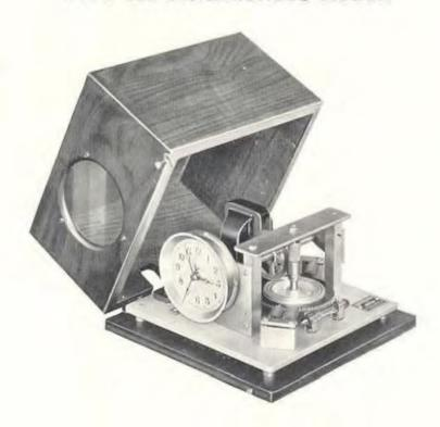
In checking a source of constant-frequency current, great accuracy may be attained by using the source to drive a synchronous motor, and counting the motor revolutions over a long period. Synchronous motors may be built which will operate properly at audio frequencies. Higher frequencies may be checked by stepping down the frequency by means of a series of oscillators, with harmonics of the lower frequency
