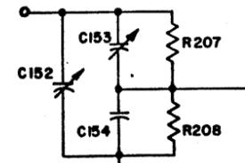
RESISTORS IN ATTENUATOR OF 33K AND BELOW ARE COMPOSITION, 25%. ALL OTHERS ARE DEPOSITED CARBON, ±1%.
