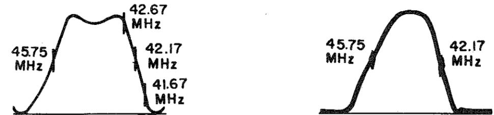
Figure 23. Typical IF curves for two types of receivers.
