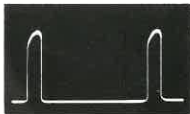
12AU7 (V15) Sync Amplifier and Clipper Plate (Pin 1) 80 Volts (PP) Horizontal.
