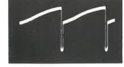
6AH4GT (V17) Vertical Output Grid (Pin 1) 85 Volts (PP) Vertical.
